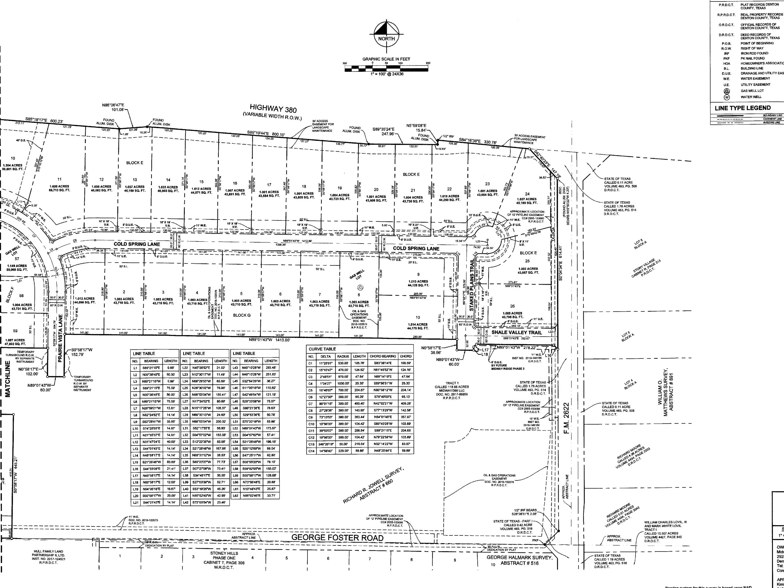
Bearing system for this survey is based upon NAD 83-Texas North Central Zone, Horizontal Adjustment to NAD 83 (1993). To convert the Surface distances to Grid values, multiply the distances by a Combined Scale Factor of 0.999880014.
